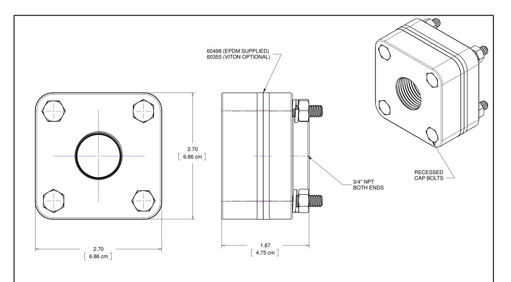
1. MATERIAL - POLYPROPYLENE, EPDM OR VITON GASKET AND 316 SS HARDWARE
